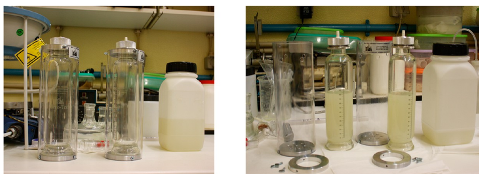
Figure 3. Glass cans used throughout this work before (left) and after addition of backbone + MEB and backbone + MMB microcapsules (right).
